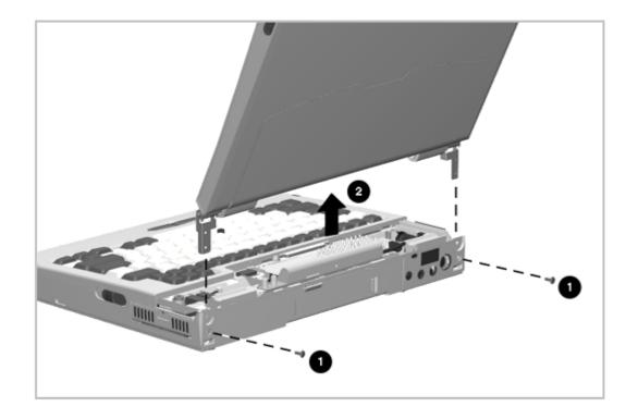
Figure 5-30. Removing the Display Assembly
